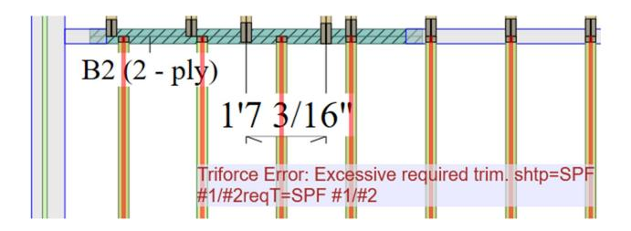
• When this error occurs, the best solution is to off-set the joists in layout so that the appropriate joist length is specified:
